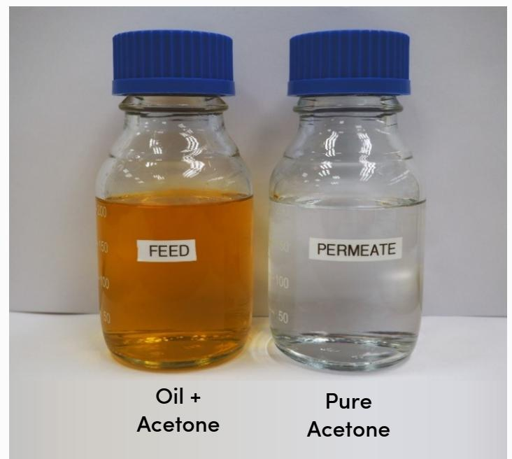
Tests performed using GreenMem® showed an average oil rejection of ~99%. The GreenMem® products archived ~15% higher oil rejections and 6 times the permeance compared to the market-leading product performed under the same conditions.
