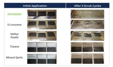
SYLVASOLV oils outperform D-Limonene, Methyl Soyate, Toluene and Mineral Spirits, in cleaning lithium complex greases after a 5 cylce, back and forth wipe. Cleaning coupons by scrub test on lithium complex greases with solvents in formulated cleaners at 5% concentration.
